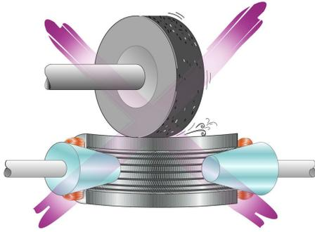
**Incorrect** clamping process
