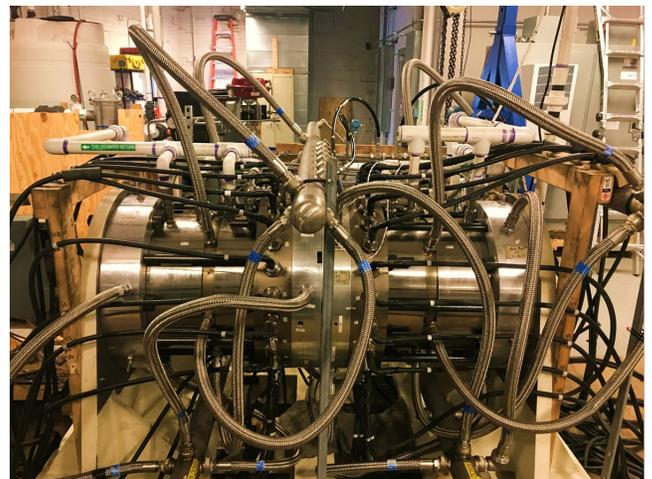
1.6MW, 25,000 RPM System for Shipboard Power Generation. Shown are two Generators configured Back-to-Back for Testing.
