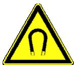
Synchronous rotors contain very powerful magnets! Ferromagnetic items, such as tools, grinding dust, cuttings, as well as tools made of ferromagnetic materials, are attracted. There is a risk of trapping fingers, resulting in injuries!
