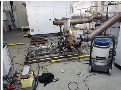
**Figure 2: Gamma Generator Hardware (Left) and Test Rig with Legacy GTE Using Fluid Film Bearing**
