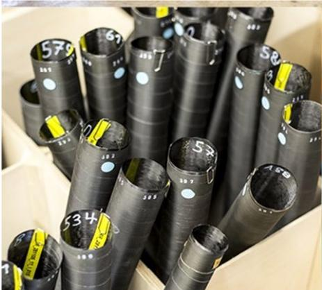
**Figure 27: Carbon Fiber Sleeve Tubes Before Being Cut to Required Lengths**
