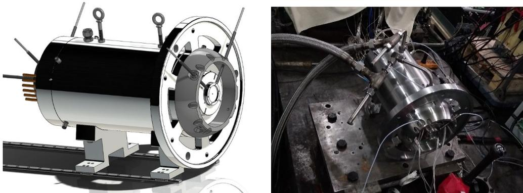
**Figure 6: 140KW Generator Test Rig: Solid Model (Left) & Actual Hardware (Right)**
