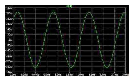
Figure 2: Ripple Current on Simulated Motor Current Waveform with Three-Level MLI & Sine Filter
